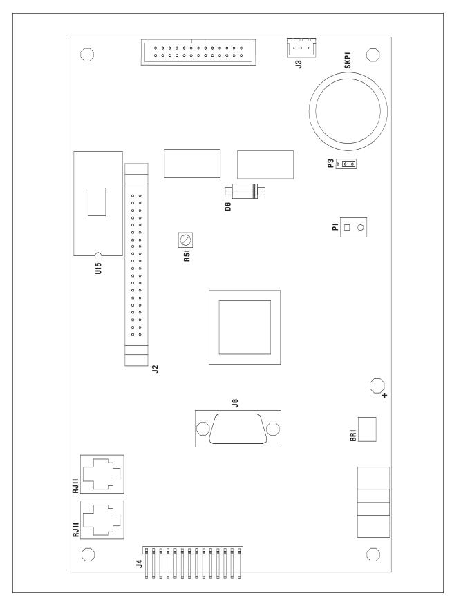
FIGURE 62: I/O Control Board and Test Point Locations
